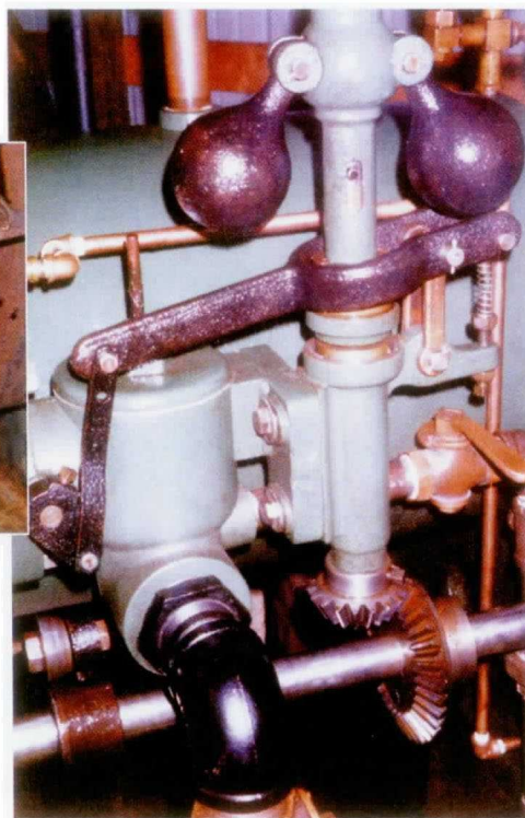
Right: The restored mixer and governor highlight the work that went into this engine's restoration. Note the new governor gears.
