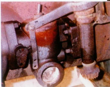
Above: Mixer and governor before disassembly.
