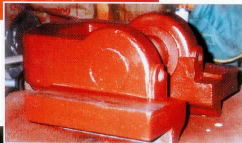
Crosshead after pouring new babbitt (above) and after a coat of primer (right). A freshly babbitted and primered bearing cap (below).
