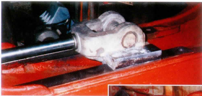
Crosshead after pouring new babbitt (above) and after a coat of primer (right). A freshly babbitted and primered bearing cap (below).
